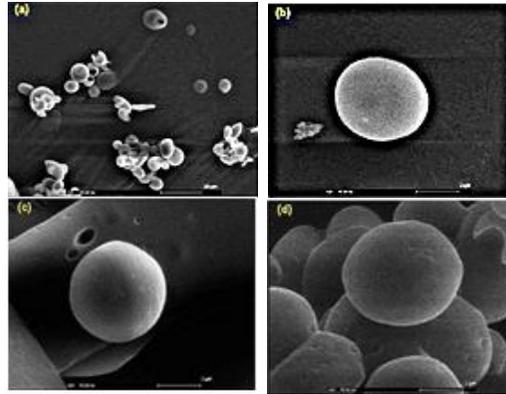
**Figure 2** Scanning electron micrographs of (a) and (b) blank calcium pectinate microparticles using 0.5% w/w pectin, (c) ibuprofen-loaded calcium pectinate microparticles using 0.5% w/w pectin and (d) ibuprofen-loaded calcium pectinate microparticles using 1.0% w/w pectin. Scale bars are shown on the individual photographs.
