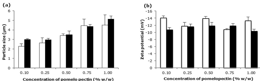
**Figure 1** Effect of concentration of pomelo pectin on (a) particle sizes and (b) zeta potentials of calcium pectinate microparticles; white columns – without ibuprofen, black columns – with ibuprofen.
