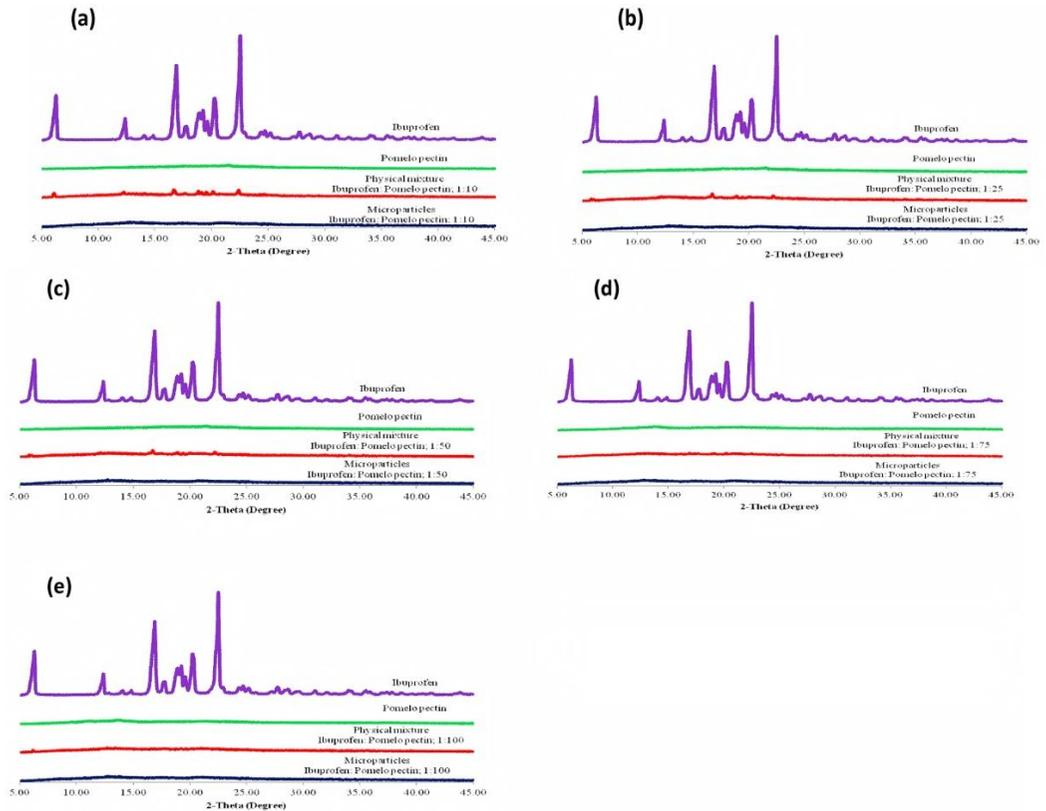
**Figure 3** Powder X-ray diffractograms of microparticles prepared from various concentrations of pomelo pectin; (a) 0.1% w/w, (b) 0.25% w/w, (c) 0.5% w/w, (d) 0.75% w/w and (e) 1.0% w/w.
